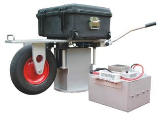
The vibrator source with active vertical vibrator kit (mounted) and additional horizontal vibrator kit (right side).
