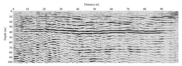
S-wave reflection seismic section.
