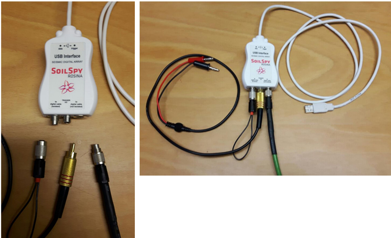
Figure 2: USB Interface with USB connection to laptop, trigger cable, cable to string and small surface end plug
