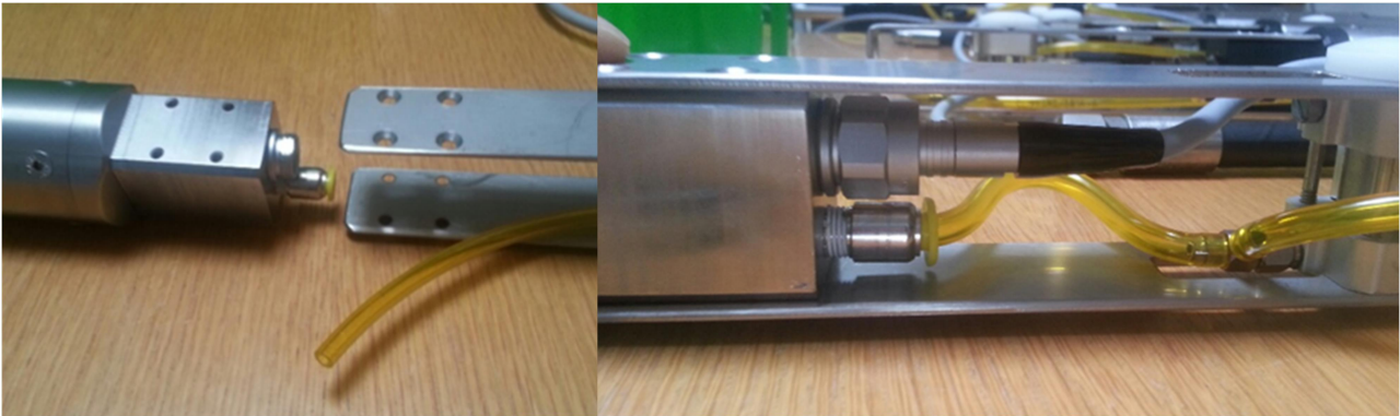
Figure 7: Screw first station to probe head
