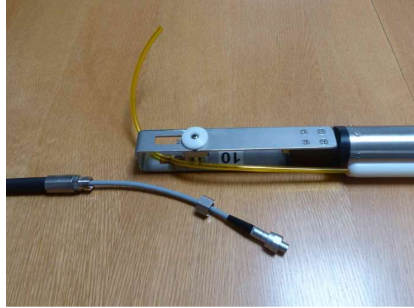
Figure 10: Put data cable trough side opening
