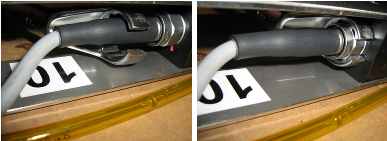
Figure 8: Connect data cable (tightly) and air hose
