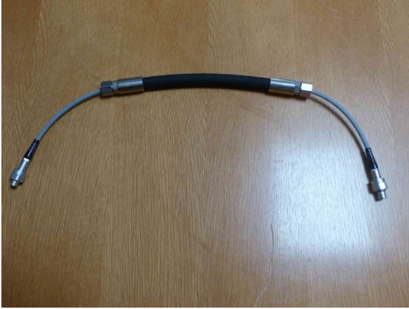
Figure 9: Station Connecting Cable
