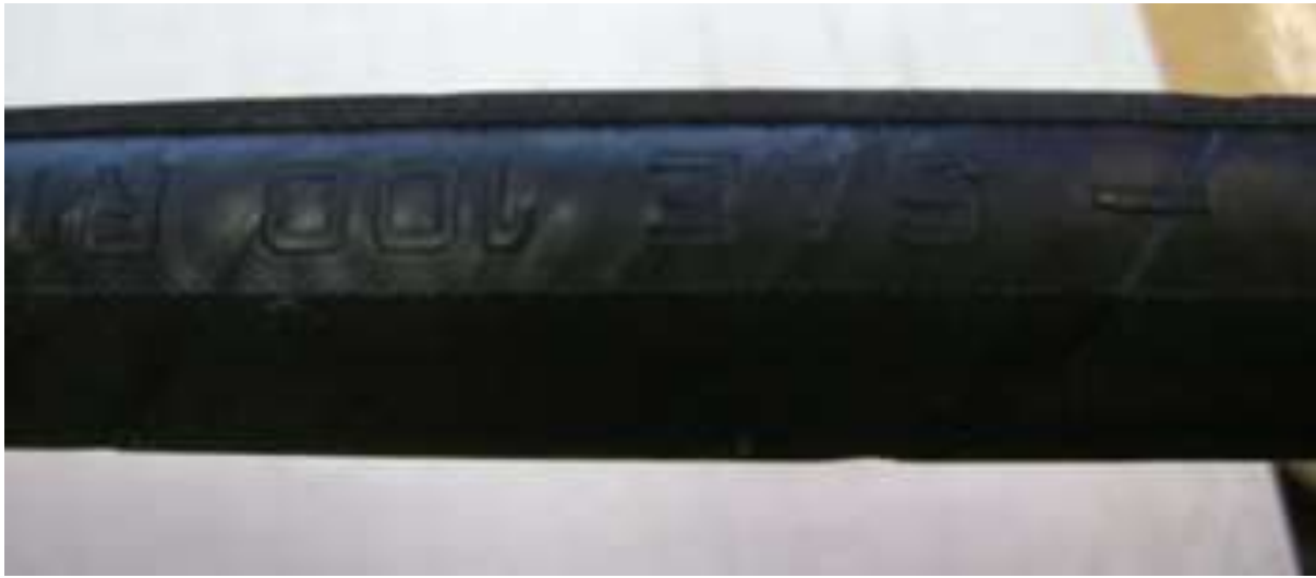
Figure 2: Marking along the rotary string is aligned to the H1 geophone
