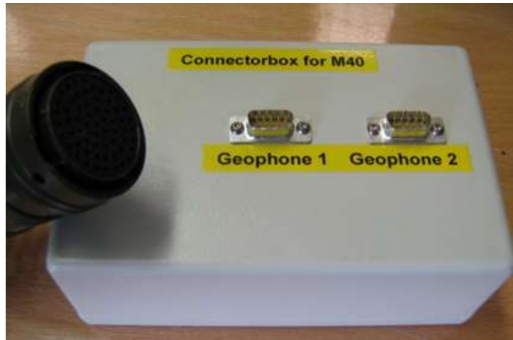
Figure 3: Connector box to seismograph (similar or different design possible for 2 x M40 units only)
