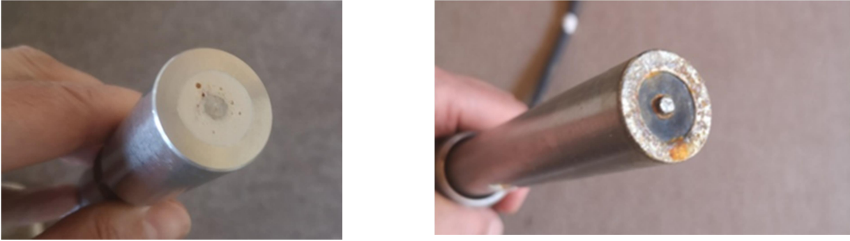
Figure 25: (left): new and flat surface of the sparker electrode (right): sparker electrode after approximately 2000 shots.
