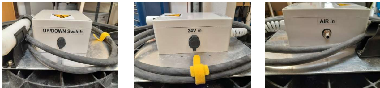
Figure 19: UP/Down remote switch box with connections
