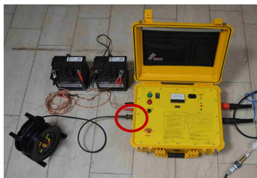
Figure 27: Connection RCU to IPG800
