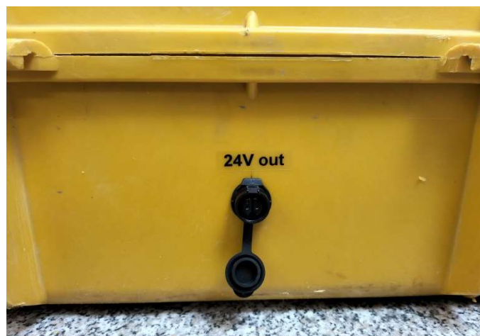
Figure 6: Rear side connector for 24V supply to the BIS-SV relay switch (2023+ IPG800 models)
