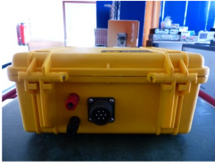
Figure 9: Rear site of RCU with banana trigger and connector to IPG5000
