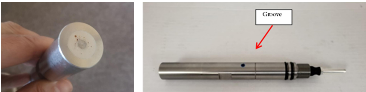
Figure 25: (left): new and flat surface of the sparker electrode; (right): sparker electrode (with groove)
