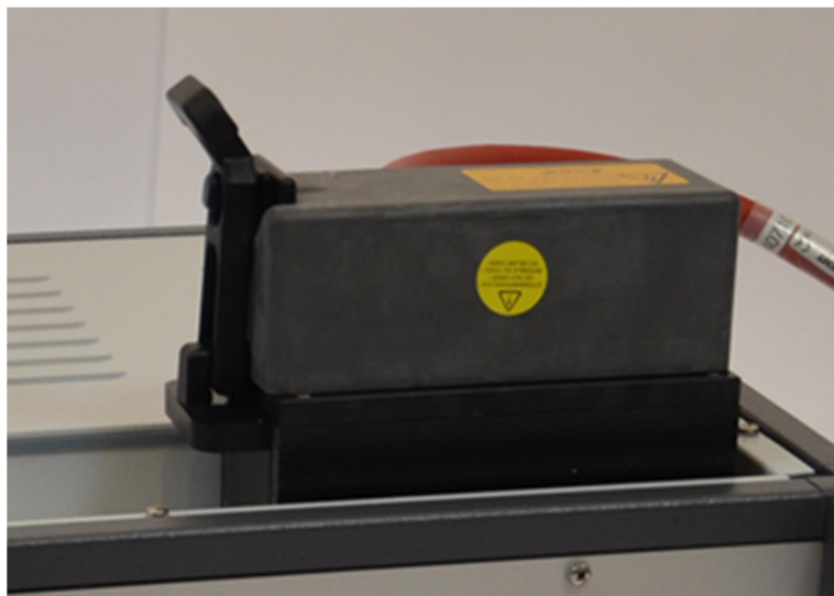
Figure 4: Rubber fixing of HV connector on IPG5000
