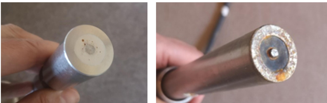
Figure 27: (left): new and flat surface of the sparker electrode; (right): sparker electrode after about 2000 shots
