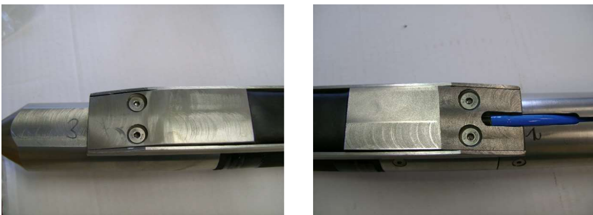
Figure 16: Unscrew to replace air bladder
