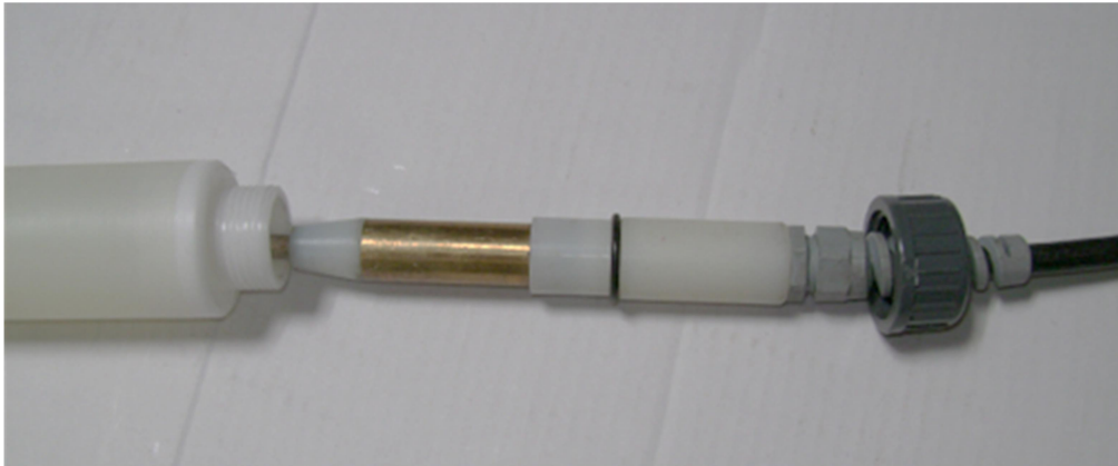
Figure 7: Connection between coaxial cable and large red HV cable on IPG5000
