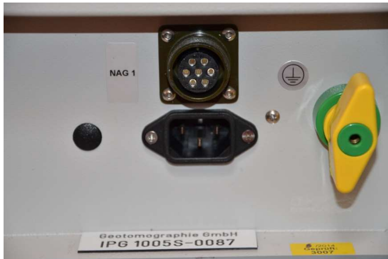
Figure 3: Details of the connecting points on the rear of the IPG5000
