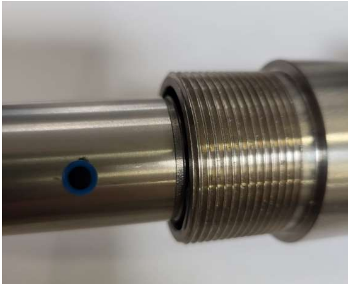
Figure 26: Sparker electrode screwed in completely
