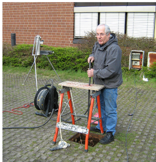
Figure 29: Fixation of the BIS-SH using the workbench
