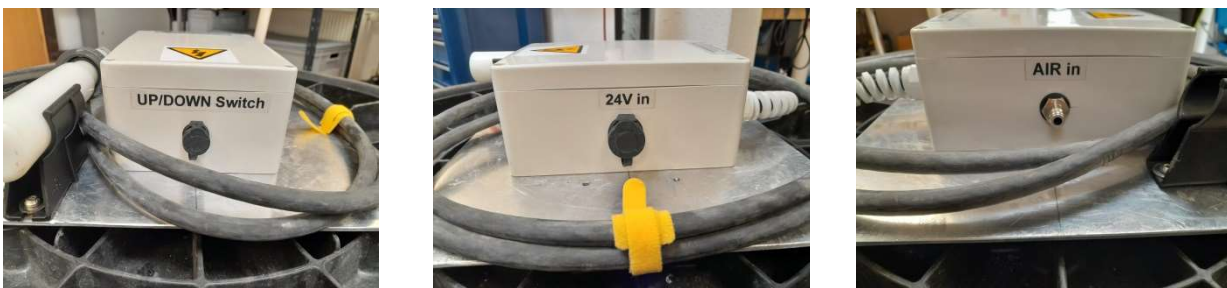
Figure 21: UP/Down remote switch box with connections
