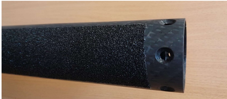
Figure 22: Friction-enhancing material covers the outer probe housing
