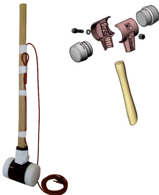
Sledge hammer with mounted piezo trigger element.
