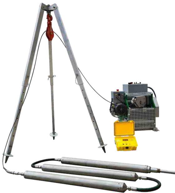
P-wave source SBS1000 with tripod, logging winch and surface control unit.
