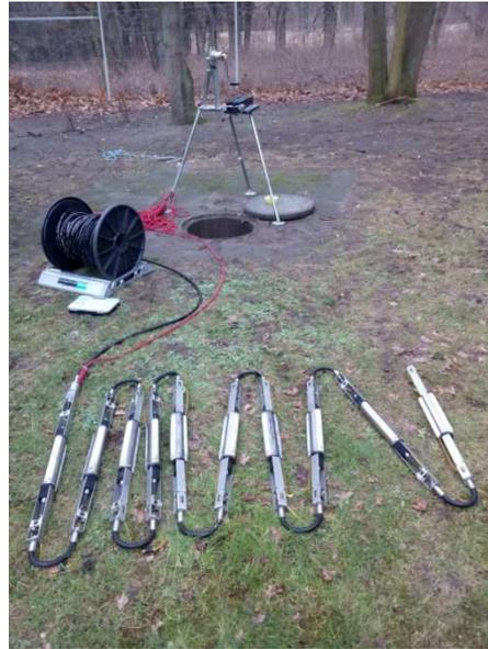
Figure 2: Prototype Multi-station Borehole Acquisition System (MBAS)
