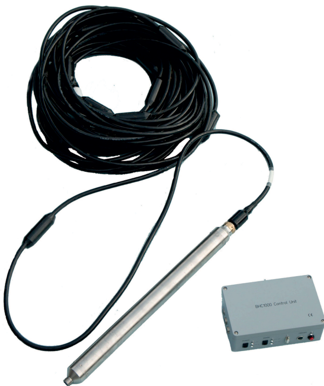
BHC1000-Sonde with BHC1000-Control Unit.
