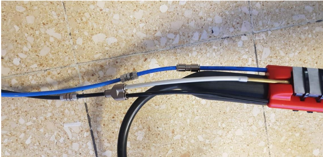
Fig. 7: Connect air hose to downhole air system
