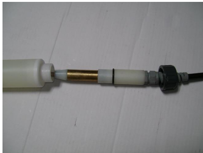
Fig. 7: Connection between coaxial cable and big red HV cable at IPG5000
