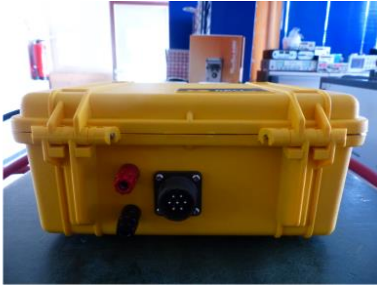
Fig. 9: Rear side of RCU with banana trigger and connector to IPG5000
