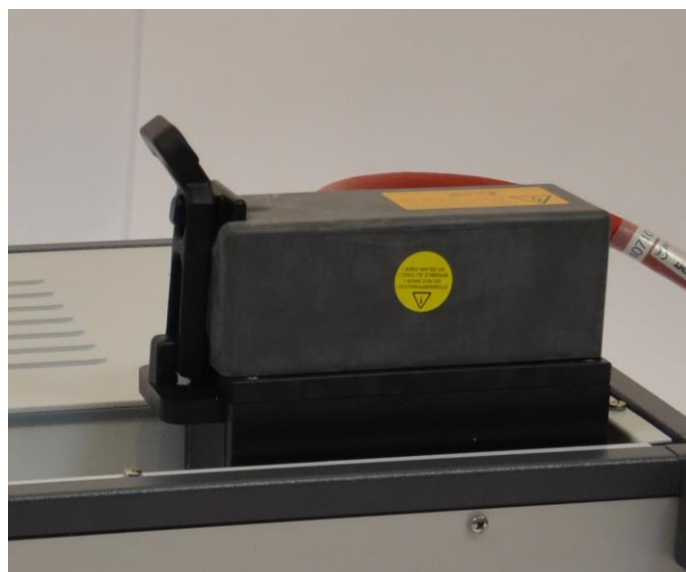
Fig. 4: Rubber fixation of HV connector at IPG5000
