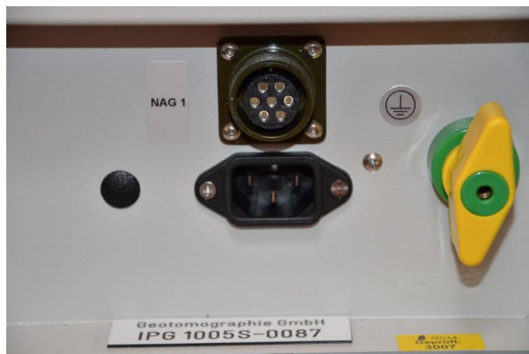
Fig. 3: Details of connecting points at IPG5000 rear side
