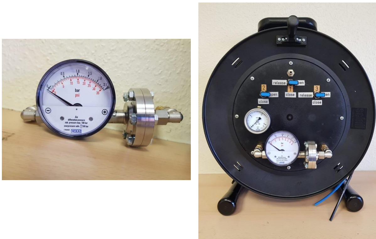
Fig. 9: Differential manometer (left) and connected to drum (right)
