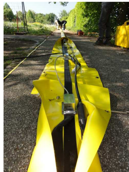
Fig. 4: Landstreamer LS-ACC with full cover protection
