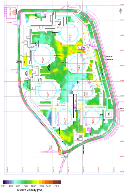
Fig 8: MASW Depth Slice at 5 m (LNG Plant Area)
